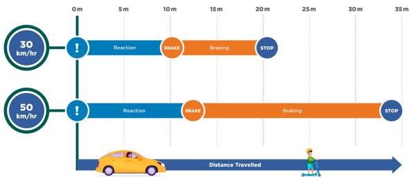
Figure 14: Driver Reaction Time and Stopping Sight Distance
